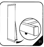
11. The unit can be leveled by adjusting the threaded feet at the bottom of the base unit.
