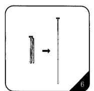
6.Unfold the pole and slip the pieces together to assemble it to a rigid pole.
