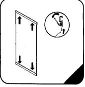
4.Open the clip bar then assemble the graphic.
