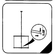
8. Take fix of the bottom pole with the special unit then spread the graphic to the top of the 3 piece pole.
